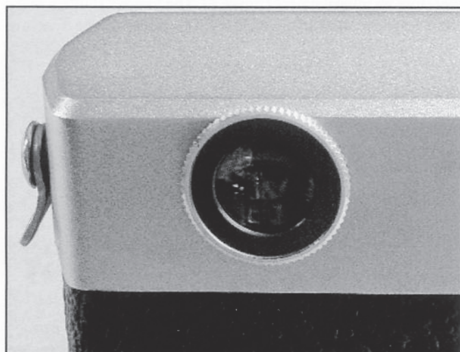
This viewfinder eyepiece, starting with Werra III, has a ring that unscrews to make a clamp for an accessory shoe and also provides a diopter adjustment. Figure 6
