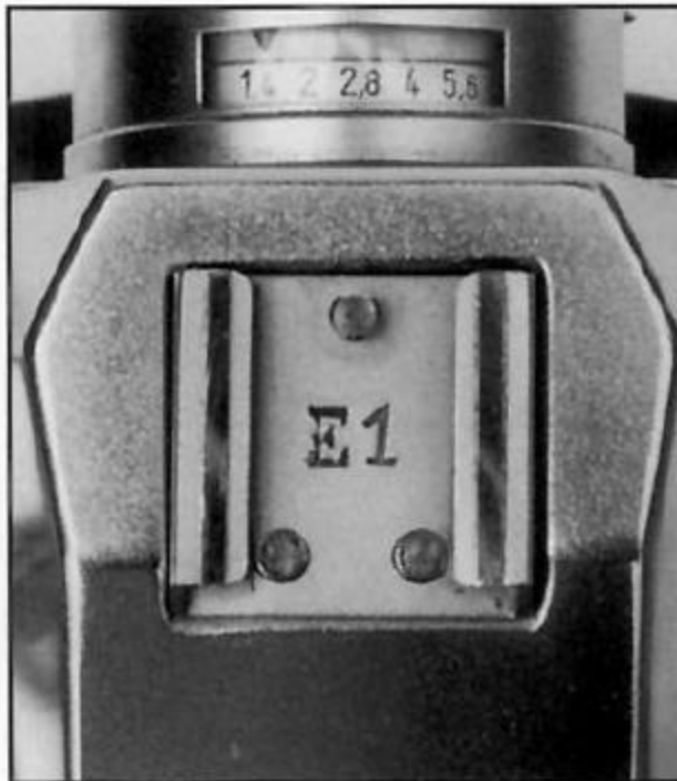
Accessory shoe of the prototype Contarex marked "E1." Figure 7
