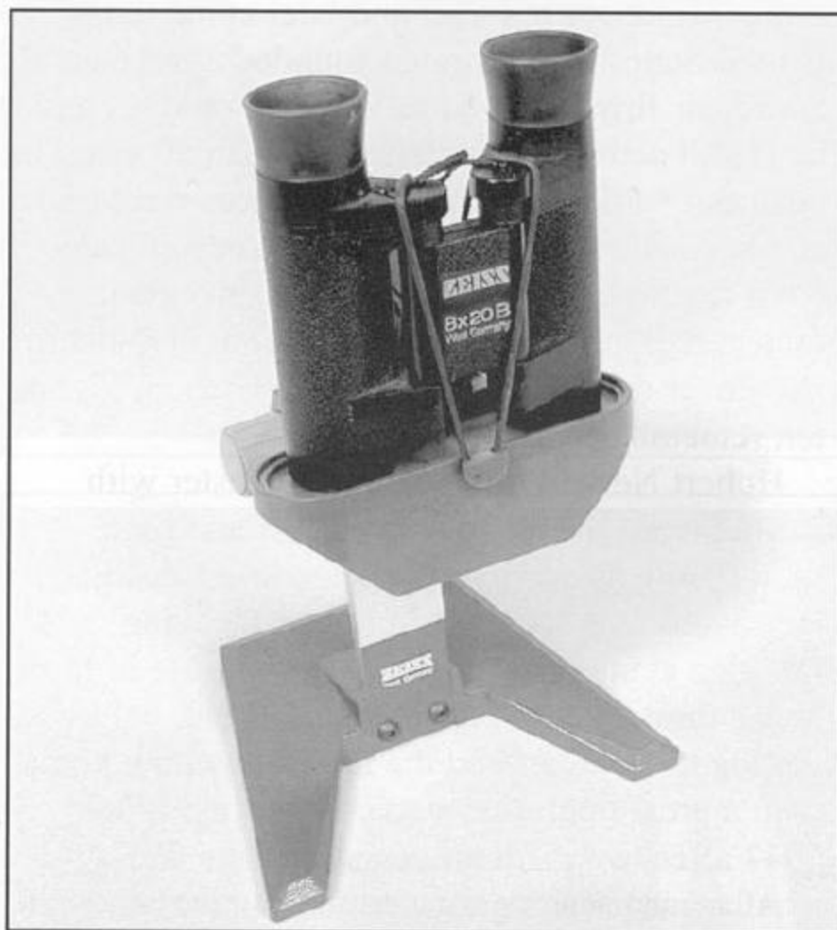
Zeiss 8 \times 20B binocular mounted on the Stereo Microscope base, left, and unmounted, right; circa 1980. The binocular is held in place with a rubber-band assembly and the base incorporates a focussing mechanism. Figure 5
