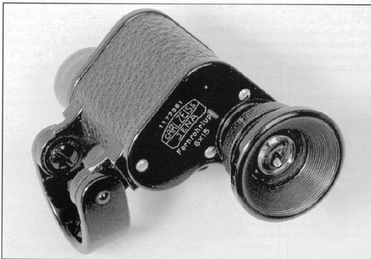
Monocular Fernrohrlupe 6x, with the close-up lens shown attached. On the right is the complete kit with handle and four close-up lenses. The monocular was manufactured in 1923. The handle allows the user to position the magnifier for best view, or to pass it to other users. Alternatively, the device could be worn like a ring by putting a finger through the loop without a handle in place. Figure 3
