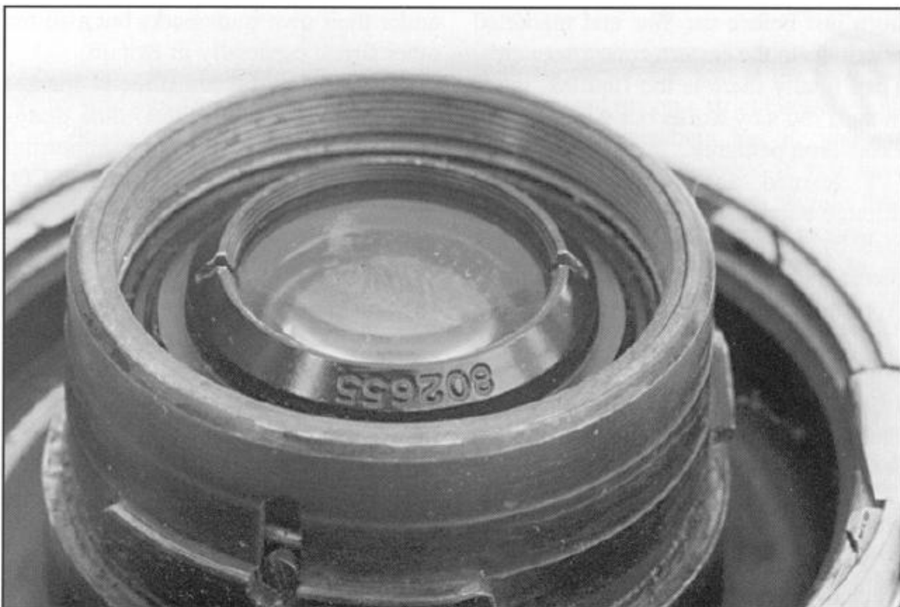
Rear view of a Biotar 3.5cm f : 2, showing the engraved six-digit number. Most Zeiss lenses, like this one, have a rear number that lacks only the "millions" digit of the full serial number.
