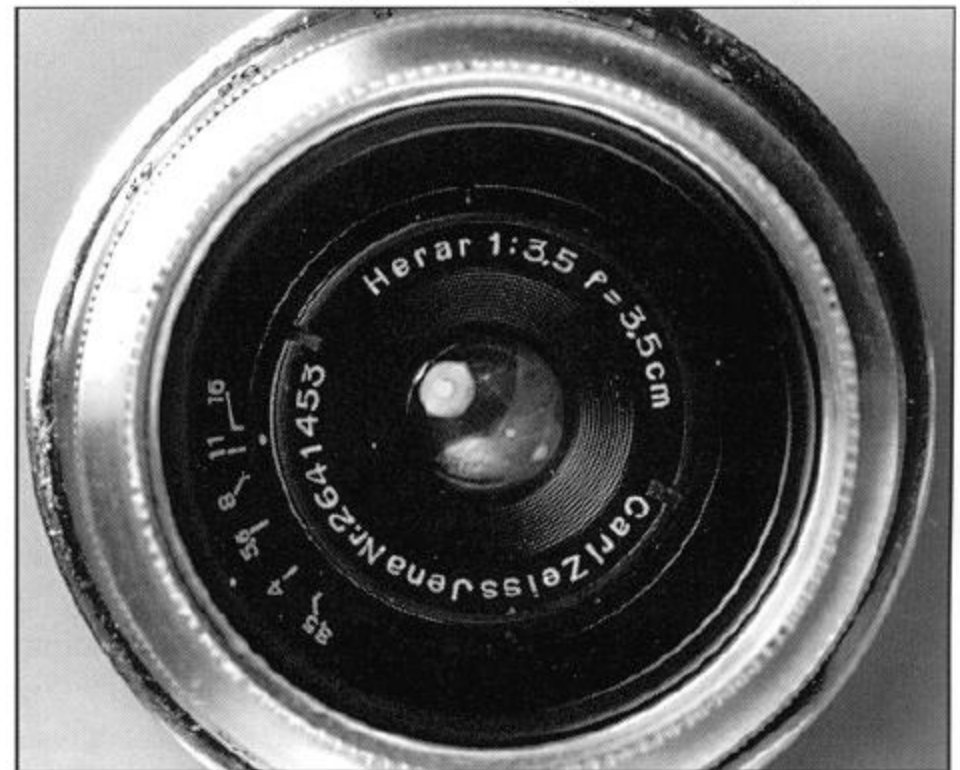
The Herar 3.5cm f : 3.5 , seen here in a close-up front view. Photo: Ghisetti
