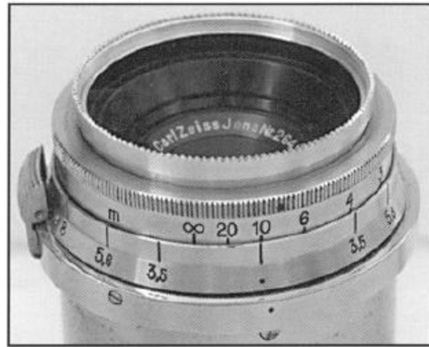
Depth-of-field scales on the three 3.5cm lenses shown on page 13. Left to right Orthometar, Herar, Biogon. Photos: Barringer
