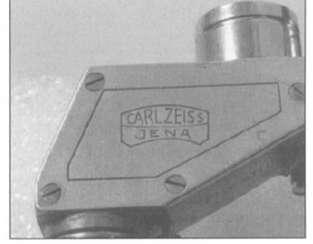
Zeiss-Marked Theatis. This Theatis from the collection of Peter Serafin is of the earliest design with small center hinge and the ability to fold completely in half for convenient storage. It was most likely painted with a textured black finish, long since lost. An interesting note is the Carl Zeiss Jena logo engraved on the prism cover. Whether this was done by Zeiss or a local distributor is open to interpretation but the example shown was manufactured prior to Zeiss' association with Möller and the lettering in the logo is just slightly different from that used by Zeiss on binoculars of that period.
