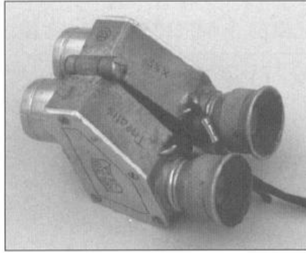
Zeiss-Marked Theatis. This Theatis from the collection of Peter Serafin is of the earliest design with small center hinge and the ability to fold completely in half for convenient storage. It was most likely painted with a textured black finish, long since lost. An interesting note is the Carl Zeiss Jena logo engraved on the prism cover. Whether this was done by Zeiss or a local distributor is open to interpretation but the example shown was manufactured prior to Zeiss' association with Möller and the lettering in the logo is just slightly different from that used by Zeiss on binoculars of that period.
