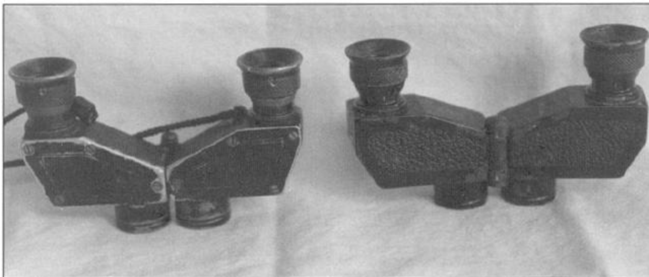
Original Möller Theatis. The first successful compact binocular design from J. D. Möller, Wedel, the Theatis, was introduced in 1920 and continued in production by Zeiss Jena until 1980. Originally finished in crinkle black enamel (left), later versions had leather inserts on the body of the binocular. From the collection of Fred Schwartzman.
