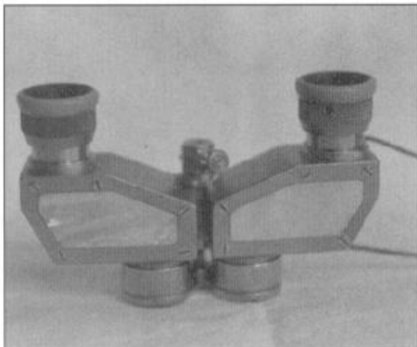
Möller Theatour. A gilt and mother-of-pearl variant of the Theatis, the 5x15 Theatour has a unique focusing system. The viewer first sets the small middle lever to the center position and then adjusts the individual eyepieces to bring the subject into focus. From that point on, the lever is used to focus both eyepieces simultaneously. The choice of the Theatour name is an obvious attempt to convey the impression that the 5x glass could be used for both theater and touring purposes. From the collection of Fred Schwartzman.
