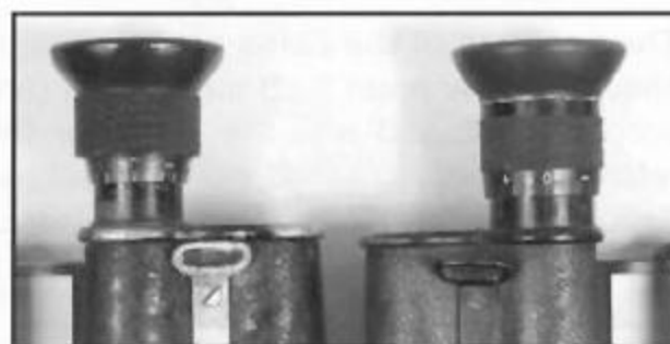
Increased body size. With the introduction of a larger body for the 4×, 6×, and 8× binoculars late in the production run, wall thickness and strength were significantly increased. These thick-walled binoculars feel significantly larger in the hand and were a precursor to the larger body sizes introduced in 1908. Top photo: a disassembled, thick-walled 6×, below, compared with an earlier thin-walled body. Bottom photo: the larger ocular tube on the right. Figure 8
