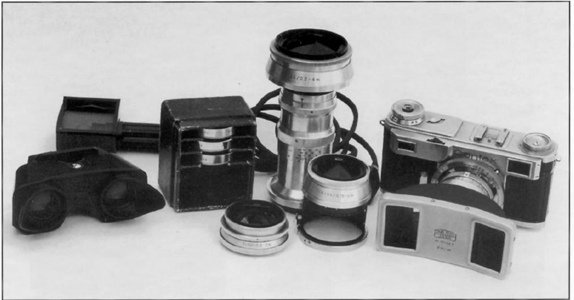
Complete stereo system from Jena. Left to right: the stereo viewer, with its illuminating system behind it; Fitted box containing three Proxars, with a space for the smaller of the two prism beamsplitters seen in front of it; Jena Contax II with the 65 mm prism attachment (marked "2-meters to infinity" but in fact good only for about 8 to 10 meters) mounted on it. At rear center is the adapter for the f/4 13.5 cm Sonnar, which is clearly much bigger than the 12 mm beamsplitter. Figure 2
