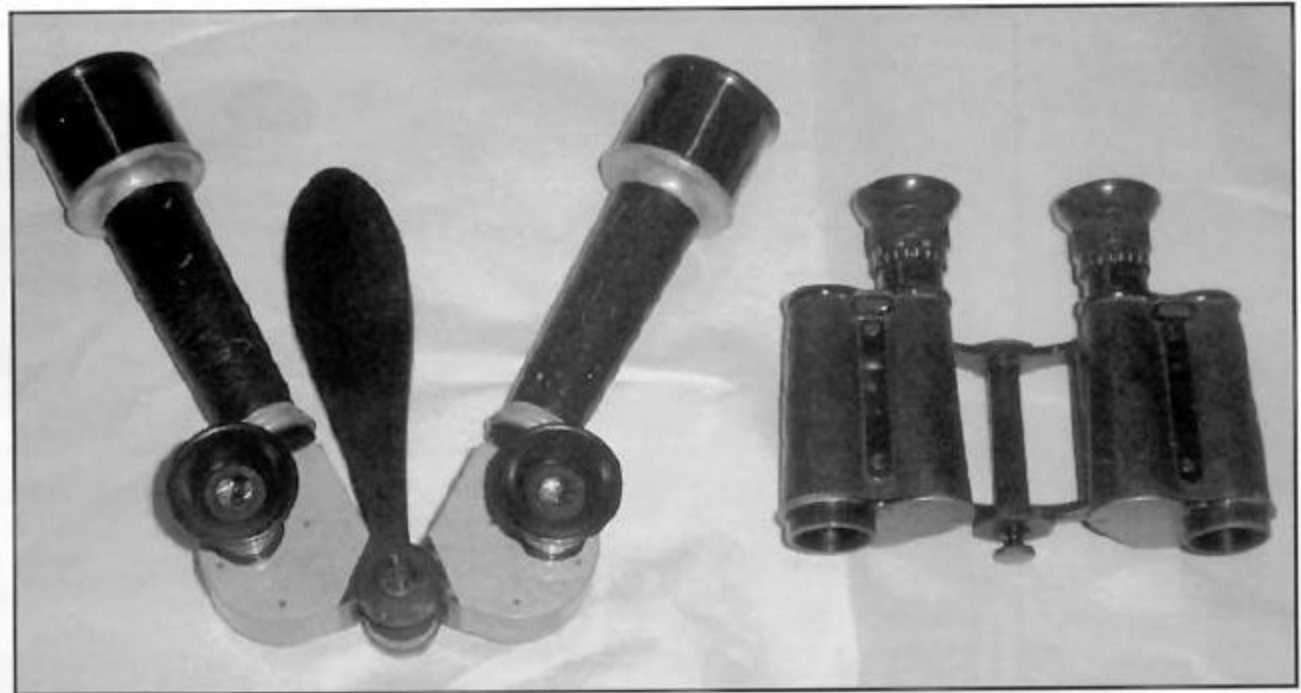
The first Zeiss binocular models consisted of three Feldstecher models and three Relief Fernrohre. Shown here is an 8x20 Relief Fernrohr, serial number 8, on the left and an 8x20 Feldstecher, s/n 7521, on the right. (Photo courtesy of Thomas Antoniadis.) Figure 3
