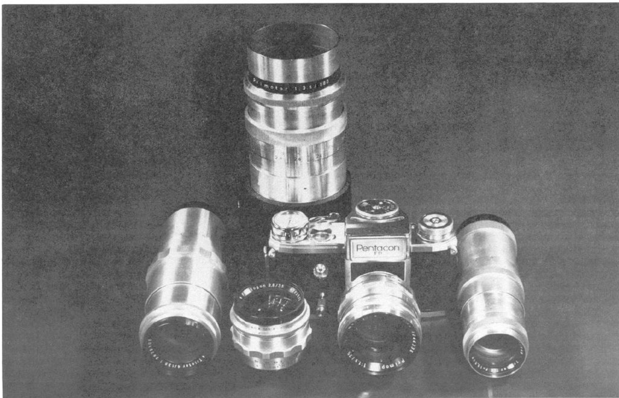
Pentacon FB with some of its lenses. An 18 cm. f3.5 Primotar is at rear. Front, left to right, are 13.5 cm. f4 Triotar, 3.5 cm. f2.8 Flektogon, 7.5 cm. f1.9 is on camera, and at far right, the 13.5 cm. f4 Triotar.
