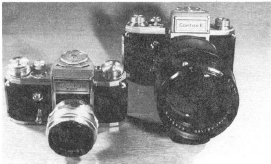
Left: Contax FBM, with auto diaphragm, meter, split image. Lens is 5.8 cm. f2 Biotar. Right: Contax E, 18 cm. f2.8 Sonnar.
