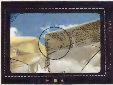
Right side of viewfinder has Exposure Indicator LEDs, with over- and underexposure warning, shutter-speed indicators. Bottom has Focus Indicator LEDs with green "in focus" dot, X for "focus not possible." Center Focus Brackets show AF sensor area.
