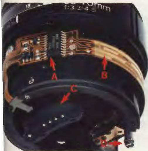
All AF Nikkors have CPU (A) connected to contact array (B) for signal exchange with camera. Zoom lenses like this also have digital switch (C) that traces focal-length setting. Steel input shaft (D) couples to camera's focus drive motor.
