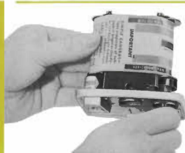
4. Secure film in empty spool slot by turning Wind Knob 3 turns. Replace camera bottom and LOCK in place.
