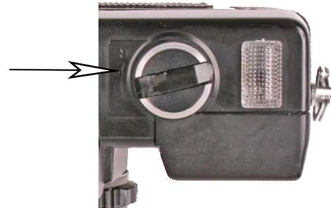
3) Once you are certain the film is rewound completely, pull up on the rewind crank until the back opens and remove the film.
