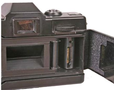
After the film is threaded into the take-up slot, advance the film by releasing the shutter and advancing the knurled knob until the film overlaps on the take up reel. Be sure the film sprocket holes are engaged in the sprockets. Now you can close the camera back. Use the knurled film advance knob to click off a few shots until the number 1 shows in the counter.
